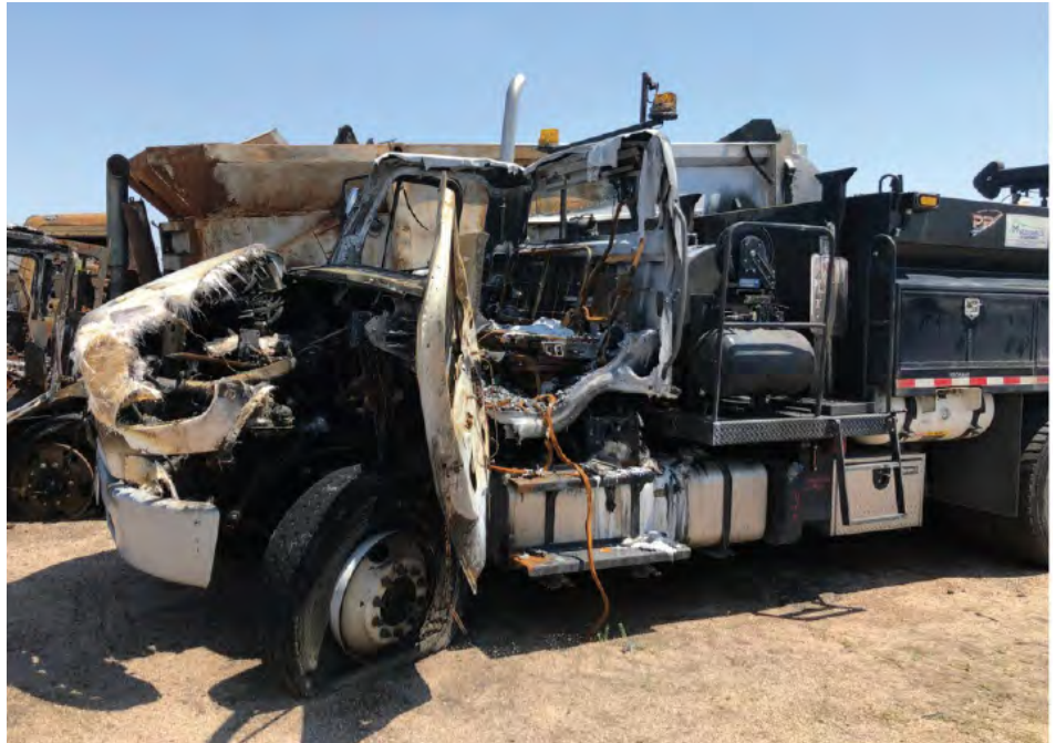
Heating with propane can be dangerous. This truck caught fire when a flameout occurred.
